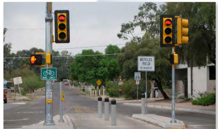
Bicycle signals: Tucson, AZ (Credit: John Holloway)
