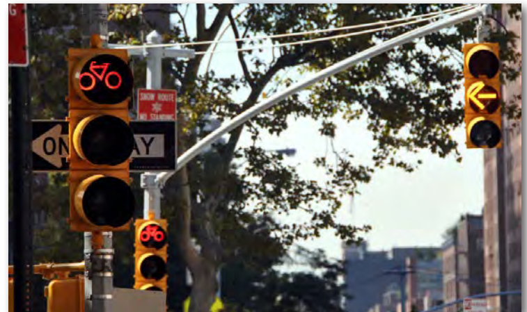
Bicycle signal head with vehicular left turn signal: New York, NY
