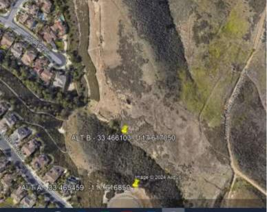
ALT B – located between a canyon. As you can see above RF Objection is not met. RF is being obstructed by the canyons to the east and west and sliver of coverage is touching only  $^{\sim}12$  homes. The elevation between the canyons is  $^{\sim}477'$  vs.  $^{\sim}626.19'$  at our proposed location. The difference between those numbers is the additional height needed to meet RF's coverage (assuming the canyons are being cleared).
