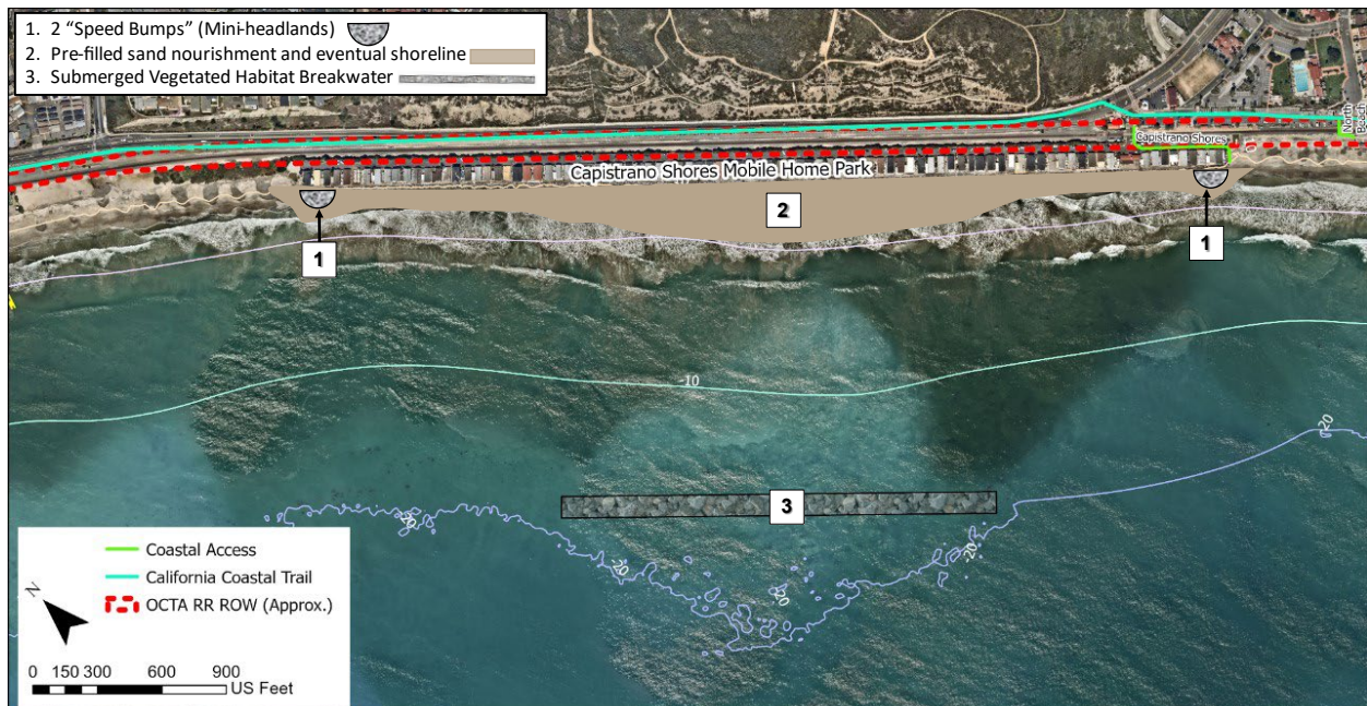
Figure 2: Conceptual Schematic for Concept 2 - Capistrano Shores Breakwater and Sand "Speed Bumps"
