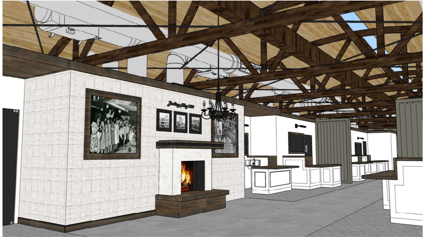
2 FOOD HALL INTERIOR VIEW 4 - PROPOSED MECHANICAL DESIGN (PRESERVES VIEW OF HISTORICAL BOW TRUSSES)
