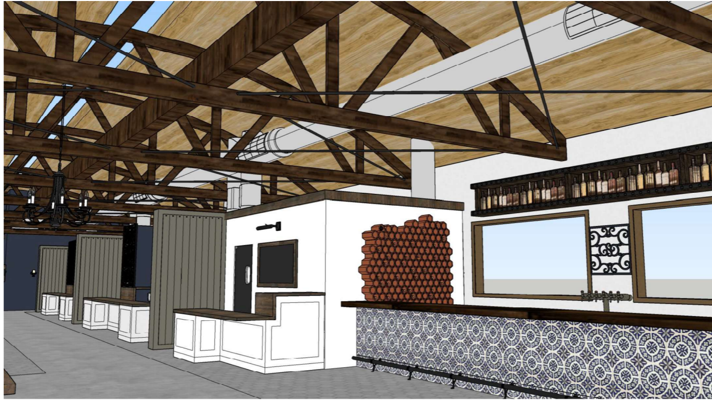
② FOOD HALL INTERIOR VIEW 3 - PROPOSED MECHANICAL DESIGN (PRESERVES VIEW OF HISTORICAL BOW TRUSSES)
