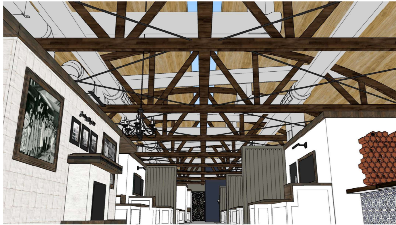
1 FOOD HALL INTERIOR VIEW 1 - CURRENTLY APPROVED MECHANICAL DESIGN (BLOCKS VIEW OF HISTORICAL BOW TRUSSES)
