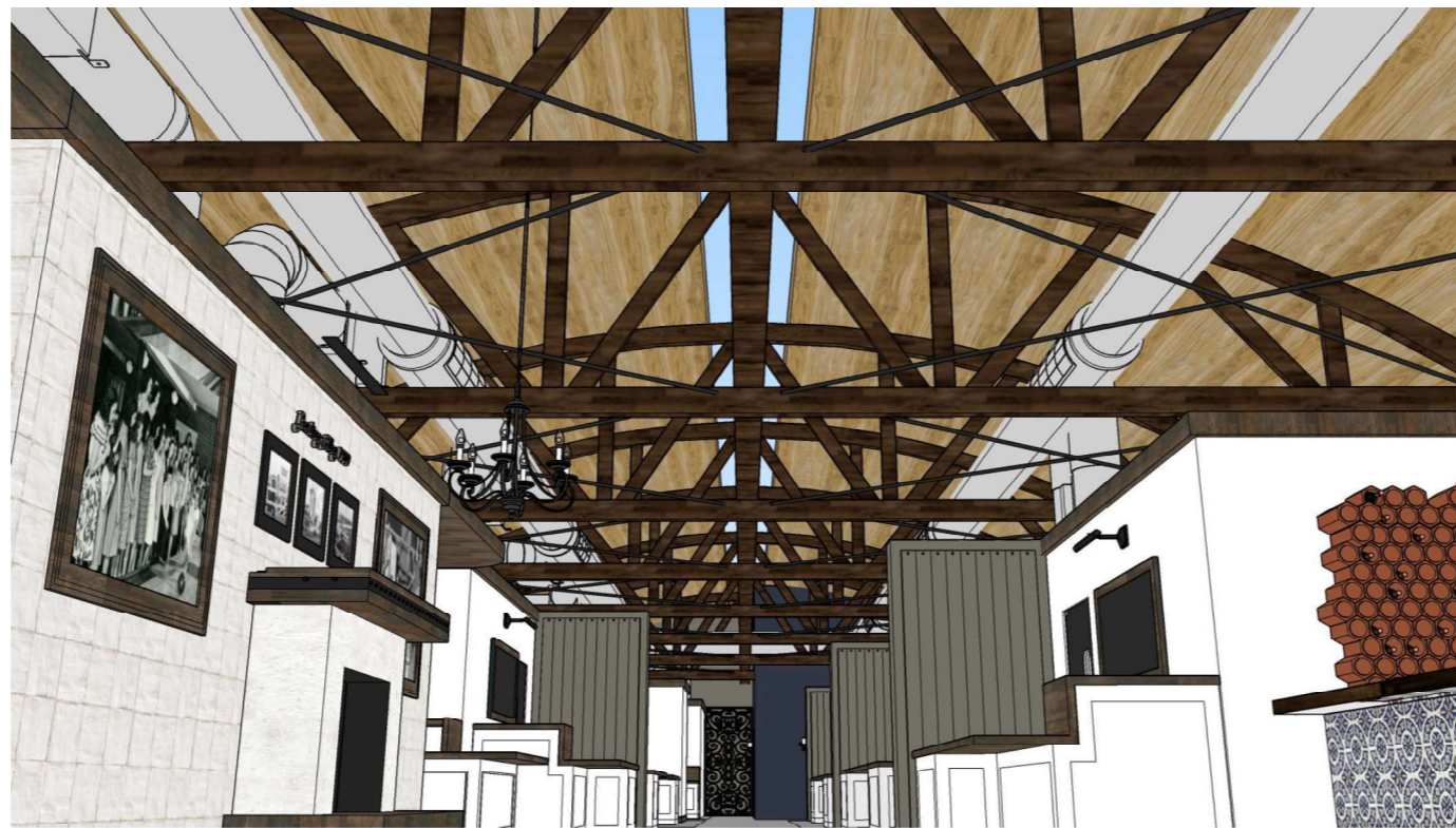
2 FOOD HALL INTERIOR VIEW 1 - PROPOSED MECHANICAL DESIGN (PRESERVES VIEW OF HISTORICAL BOW TRUSSES)
