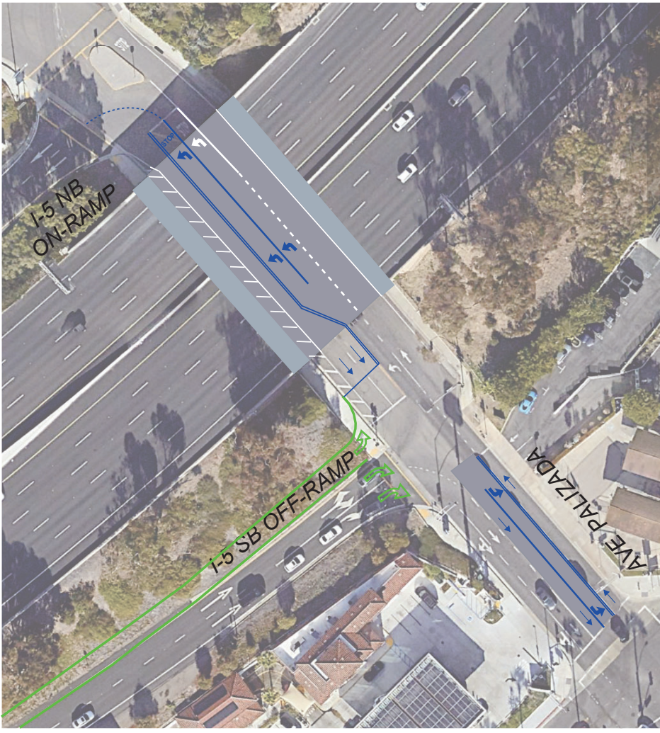
POTENTIAL STRIPING ON AVE PALIZADA BETWEEN I-5 NB ON-RAMP AND SB OFF-RAMP WITH ADDITIONAL SB OFF-RAMP LANE
