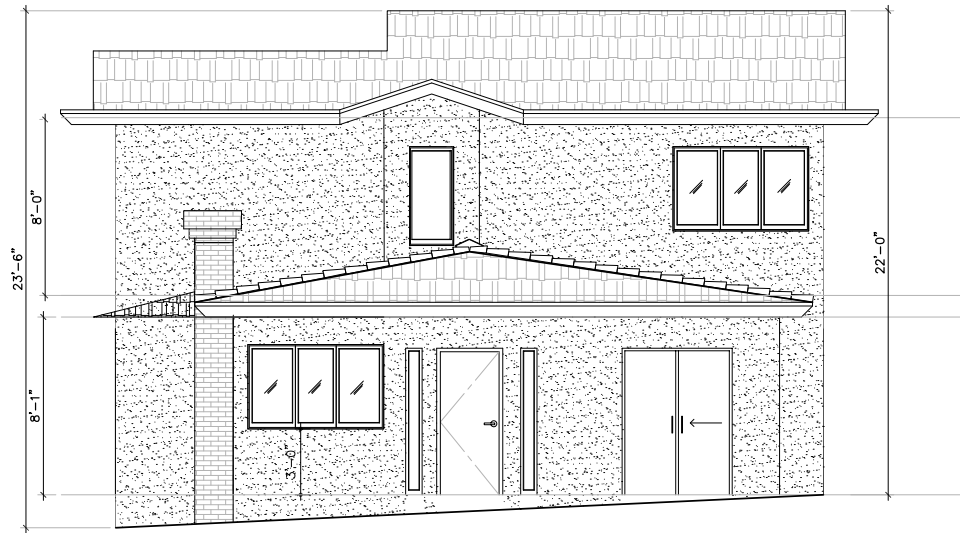
FRONT ELEVATION (EXISTING)
