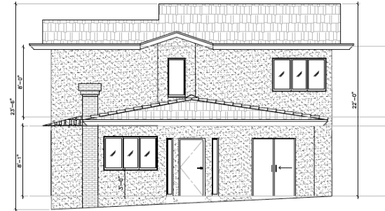
FRONT ELEVATION (EXISTING)
