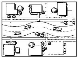
Chicanes are sometimes called deviations, serpentines, reversing curves and twists. Chicanes are curb extensions that alternate from one side of the street to the other, forming S-shaped curves. Chicanes can also be created by alternating on-street parking, either diagonal or parallel, between one side of the street and the other. Each parking bay can be created either by restriping the roadway or by installing raised, landscaping islands at the ends of each parking bay.
