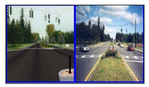
A gateway is a special entrance that reduces the width of a travel way, often implementing the use of islands. It is usually placed in a roadway to define the entry to a residential area and/or to narrow each direction of travel and interrupt the view path along the center of the roadway.
