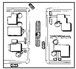
Mid-block medians are sometimes referred to as center island narrowing, median slow points, or median chokers. Raised islands located along the centerline of a street that narrow the travel lanes at that location
