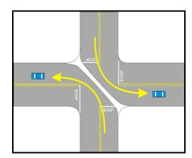
Diagonal road closures are closed to motor vehicles but traversable by pedestrians and bicyclists. A barrier placed diagonally across a four-legged intersection, interrupting traffic flow across the intersection.
