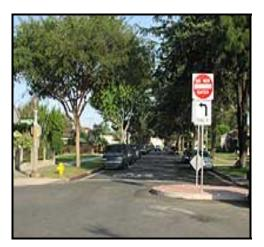
Semi-diverters are extensions from the curb or islands - usually extending from a corner of an intersection that block one directional lane of the street.
