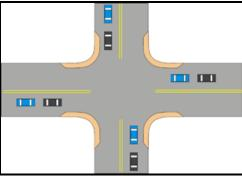
Neck downs, also known as nubs, bulbouts, knuckles, intersection narrowings, corner bulges, and safe crosses. Neck downs are curb extensions at intersections that reduce the roadway width from curb to curb. They "pedestrianize" intersections by shortening crossing distances for pedestrians and drawing attention to pedestrians via raised peninsulas. They also tighten the curb radii at the corners, reducing the speeds of turning vehicles.
