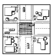
These are raised areas, which cover the entire intersection. They have ramped edges on all approaches and exits and can incorporate textured paving materials on the flat section.
