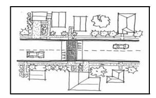
Raised crosswalks are Speed Tables outfitted with crosswalk markings and signage to channelize pedestrian crossings, providing pedestrians with a level street crossing. Also, by raising the level of the crossing, pedestrians are more visible to approaching motorists.
