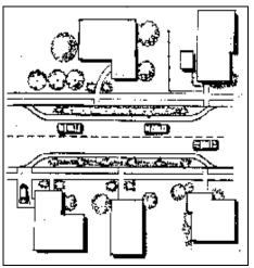
Curb extensions at midblock or intersection corners that narrow a street by extending the sidewalk or widening the planting strip
