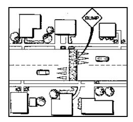
Speed humps are rounded raised areas placed across the roadway. They are generally 10 to 14 feet long (in the direction of travel), making them distinct from the shorter "speed bumps" found in many parking lots, and are 3 to 4 inches high. The profile of a speed hump can be circular, parabolic, or sinusoidal. They are often tapered as they reach the curb on each end to allow unimpeded drainage.
