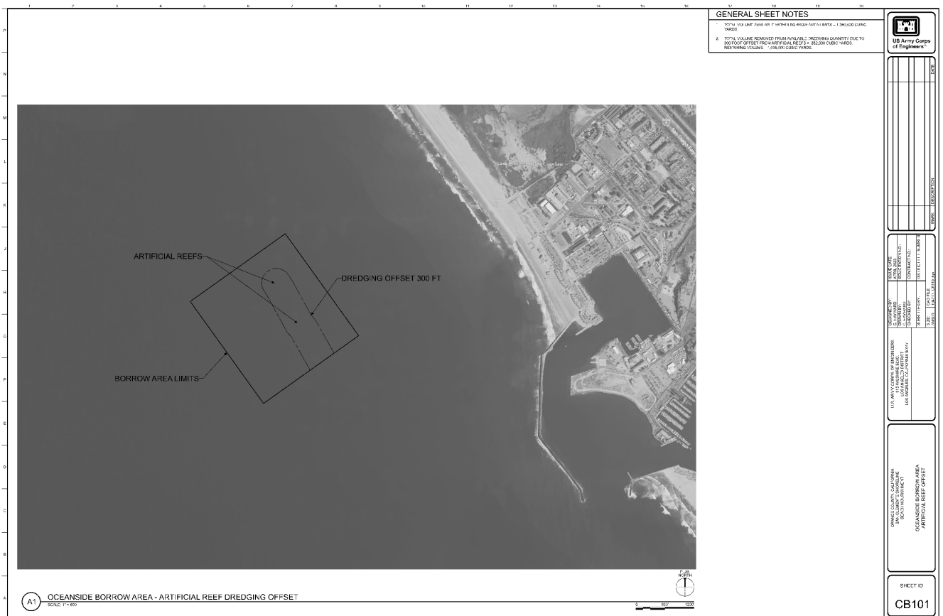
Figure 2. Updated Borrow Site schematic with 300 foot dredging offset depicted for CDFW Artificial Reef 2 avoidance.
