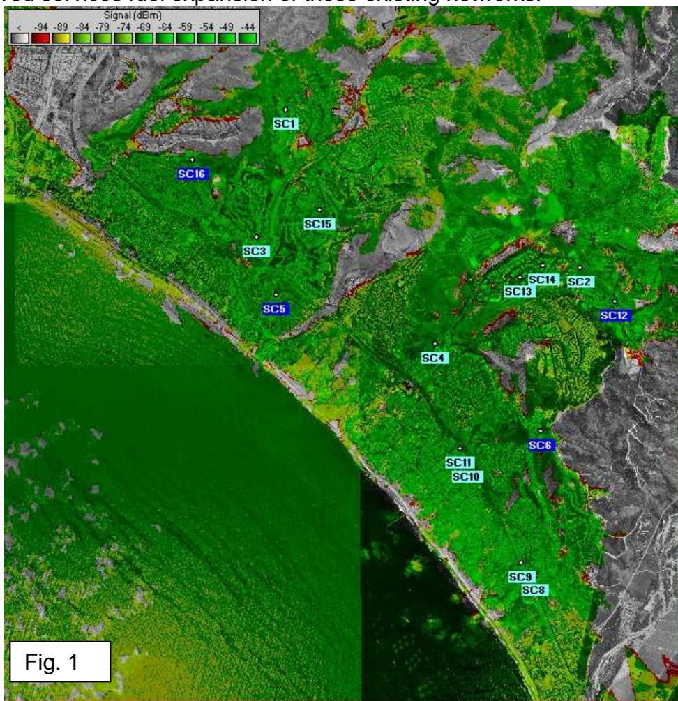
Figure 1 shows the existing wireless footprint of the combined coverage of all carriers in San Clemente. Municipal owned properties are labeled in dark blue.
