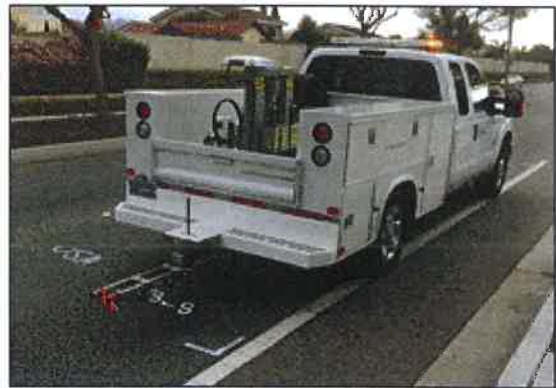
Figure 10 – Falling Weight Deflectometer
