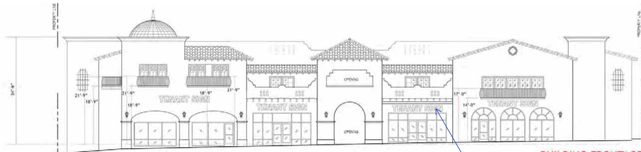
CALVADA DEVELOPMENT TENANT SIGNAGE - FULL NORTH ELEVATION WALL SIGN - TENANT STANDARD SCALE: 1/16" = 1'-0"
