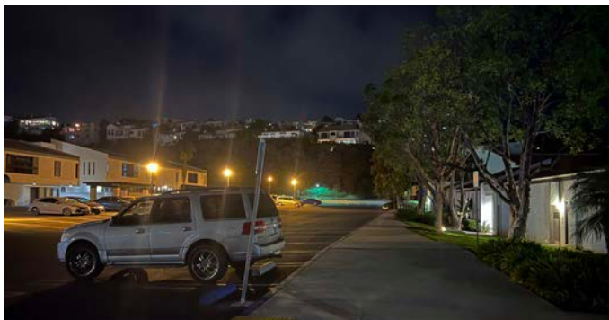
Photo 17: Bright high pressure sodium parking lot lights (≈4-6 fc)
