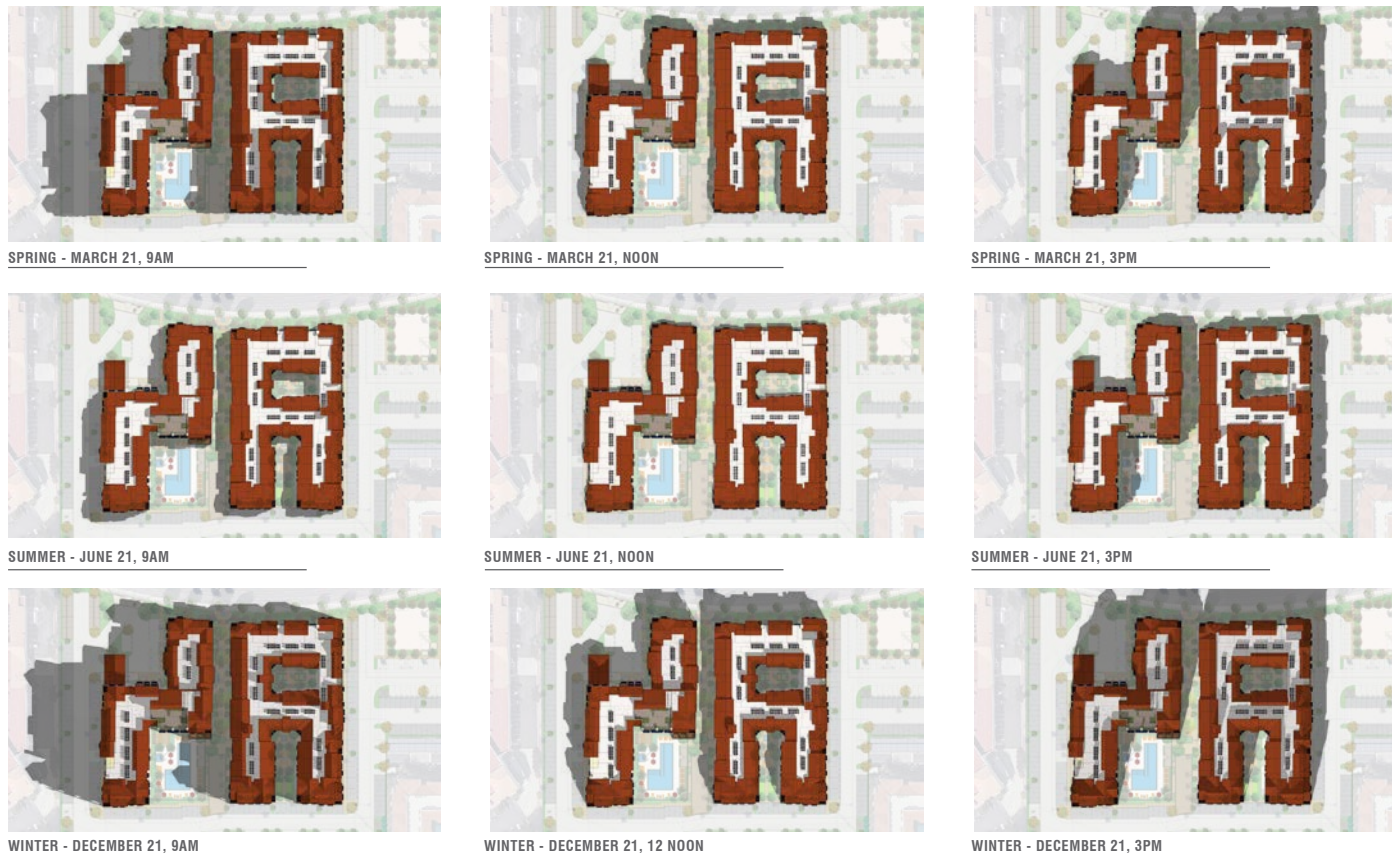
FIGURE 25: Proposed shade and shadow conditions (north is up, I-5 is along the south at the bottom of each diagram)
