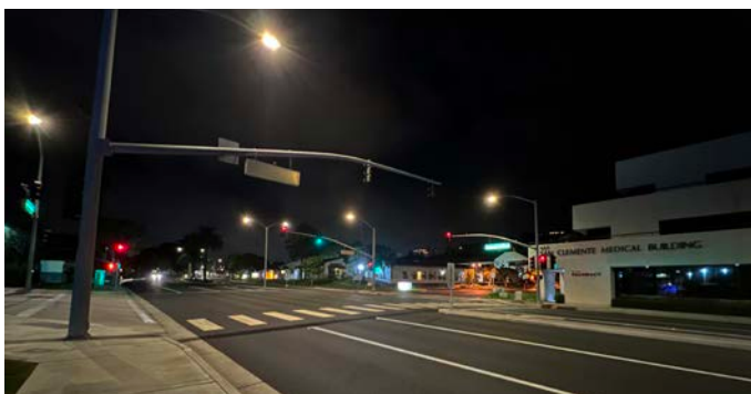
Photo 11: North on Camino de los Mares near Sr. Housing ( \approx 1-2 fc)
