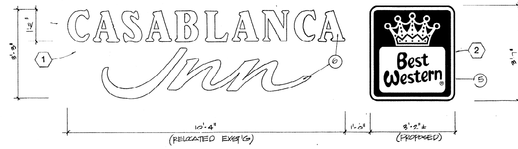
GABLE SIGN (A) 3/4"=1'-0" A NEW SIGN UTILIZING EXISTING, RELOCATED CHANNEL LETTERS AND A NEW LOGO.
