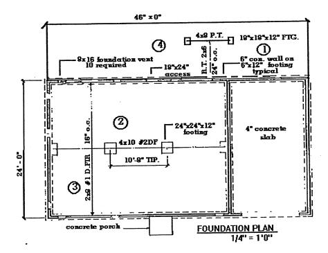
The foundation plan is a detailed drawing of the foundation, as seen from above. Suggested scale is 1/4"=1'0", with dimensions and other important information, including:
