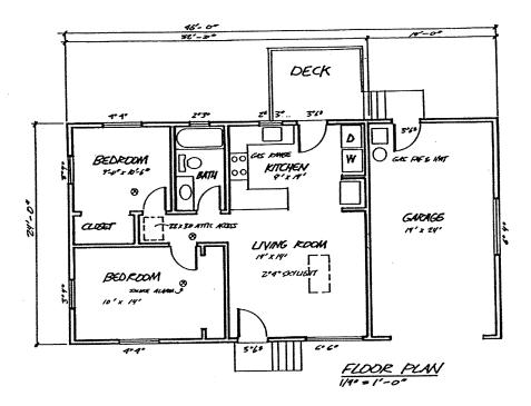
The floor plan is a detailed "map" of the new work in your project, and sometimes parts of the existing building, too. We suggest you use the scale 1/4"=1'0", and include the following:
