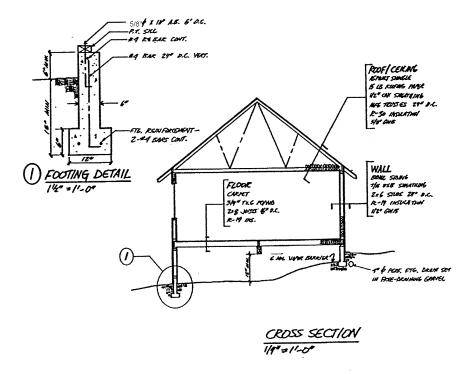
A cross section is a handy way to show lots of information. It's like slicing through an apple to see the core inside. A good scale to use is, again, 1/4"=1'0", and a complete cross section would include:
