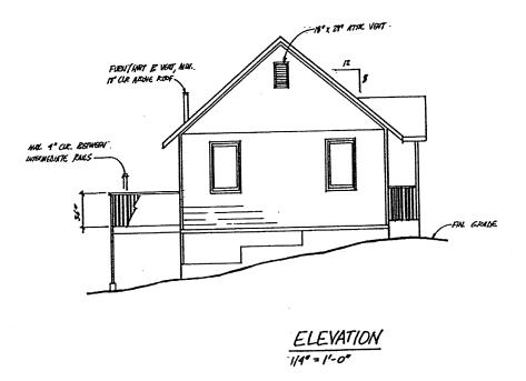
Elevations show what the building will look like from its exterior. Recommended scale is 1/4"=1'0". Depending on the specific project, sometimes just one elevation (like the "north" side, for example) is sufficient. For other more complex projects, views of the north, east, south and west sides must be shown, including:
