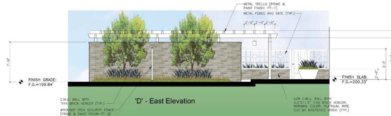
3 EMERGENCY GENERATOR ENCLOSURE - ELEVATIONS
