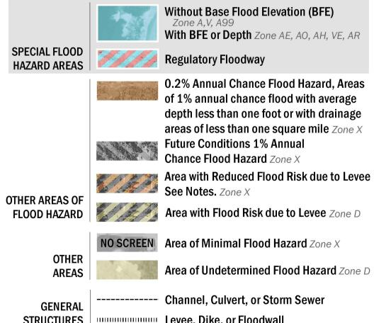
STRUCTURES Levee, Dike, or Floodwall 18.2 Cross Sections with 1% Annual Chance 17.5 Water Surface Elevation 8 ---- Coastal Transect —--- Coastal Transect Baseline --------- Profile Baseline - Hydrographic Feature **Base Flood Elevation Line (BFE)** Limit of Study OTHER **Jurisdiction Boundary FEATURES**
