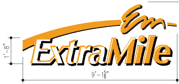
EXTRA MILE CHANNEL LETTERS 27.8 sq. ft. NEW INTERNALLY LED ILLUMINATED (SEE SECTION)
