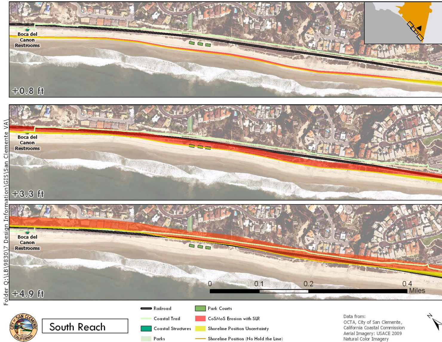
Figure 23: Shoreline Erosion Hazards, South Reach, San Clemente (1 of 2)
