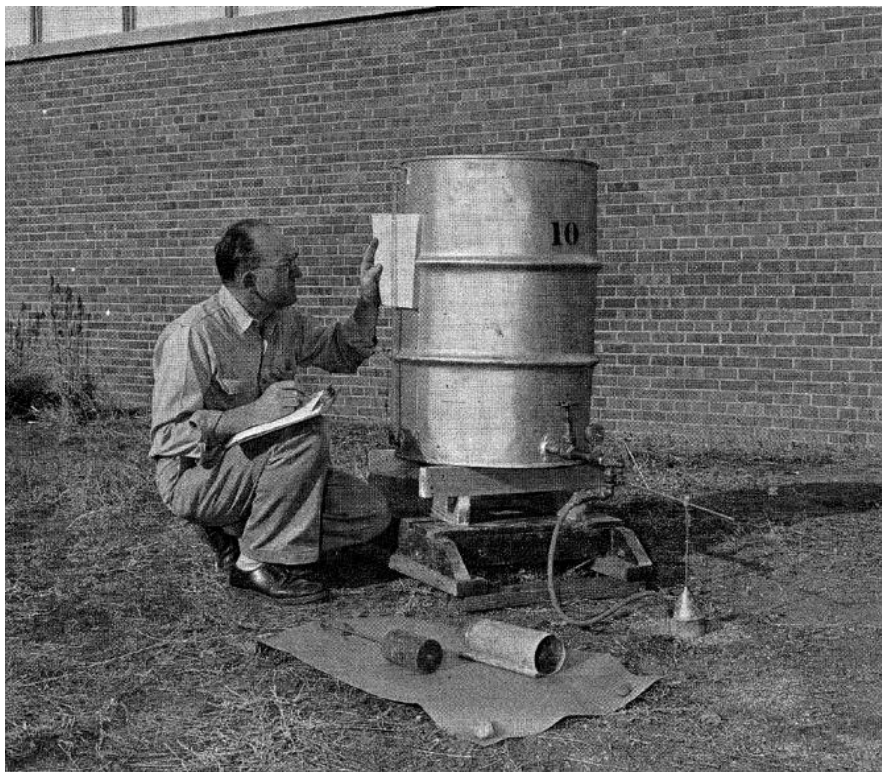
Figure VII.13. Typical Well Permeameter Test Installation
