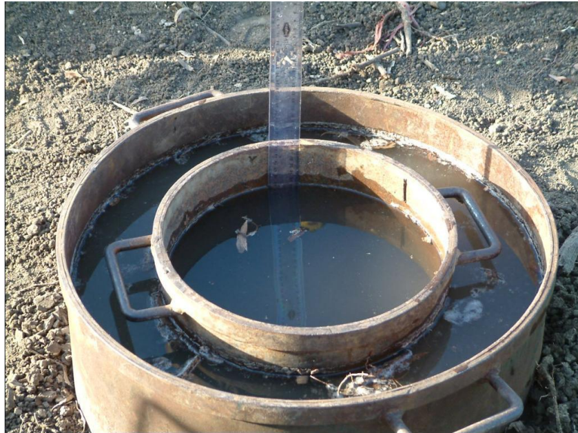
Figure VII.5. Photo of Simple Double Ring Infiltrometer
