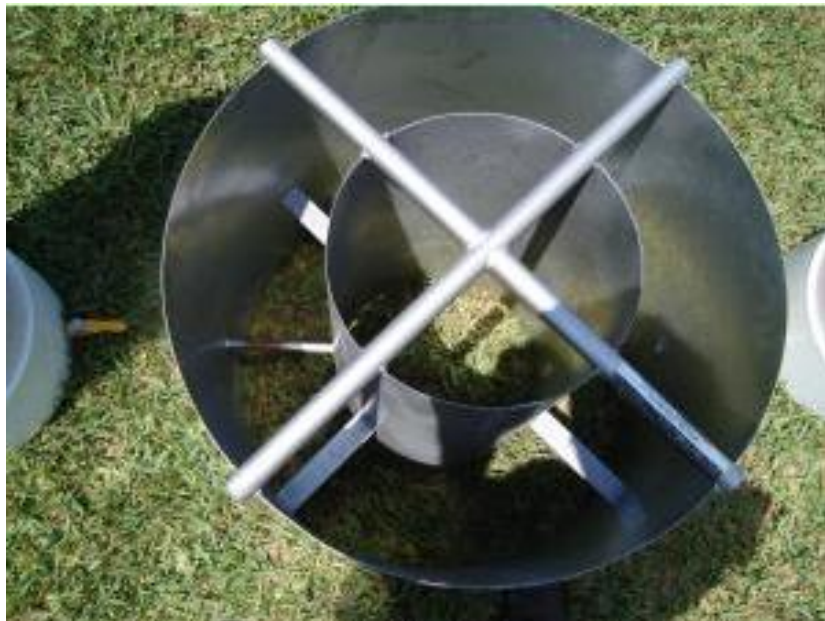
Figure VII.6. Photo of Pre-fabricated Double Ring Infiltrometer
