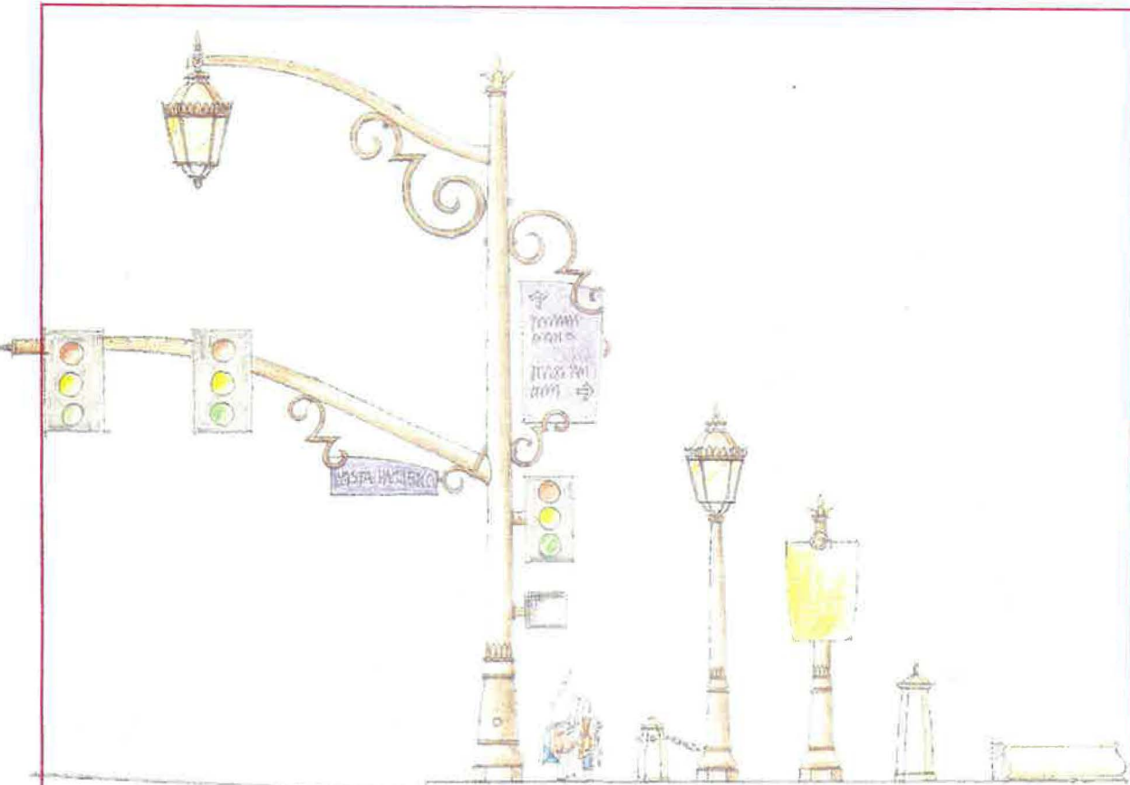
STREETLIGHT STANDARD BOLLARD PEDESTRIAN LIGHT STANDARD SIGN POST MARKER PIER PRECAST LOW WALL
