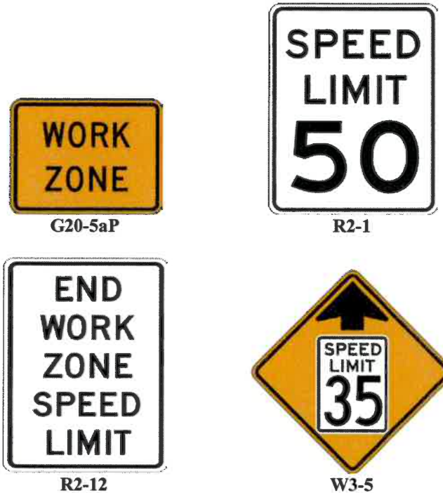
Figure 2-5: Temporary Traffic Control Regulatory Signs
