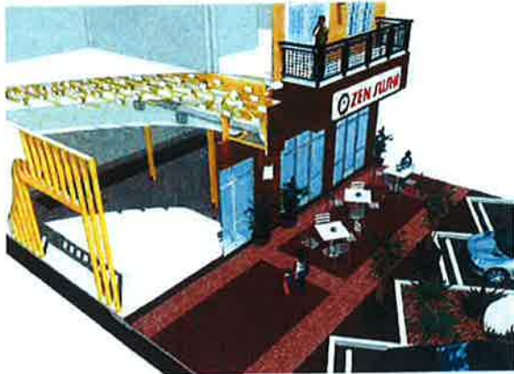
Architects used strategically placed engineered wood beams and columns to create open and flexible retail spaces within the modules while significantly reducing construction costs. (JHP)
