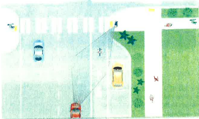
Curb extensions (Credit: Michele Weisbart)
