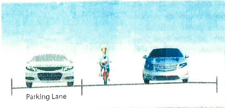
Shared roadway (Credit: Michele Weisbart)
