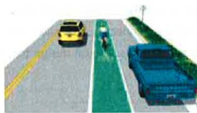
Colored bike lanes enhance the visibility of cyclists on bike lanes the bike lanes themselves. Color can be applied to the entire bike lane or at high-risk locations where motorists are permitted to merge into or cross bike lanes. This application is not yet approved by the CA MUTCD.
