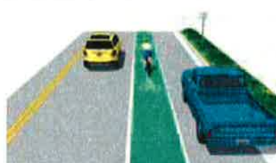
Colored bike lanes enhance the visibility of cyclists on bike lanes the bike lanes themselves. Color can be applied to the entire bike lane or at high-risk locations where motorists are permitted to merge into or cross bike lanes. This application is not yet approved by the CA MUTCD.
