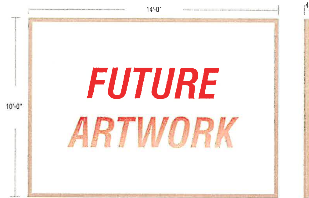
F NEW SINGLE FACED NON-ILLUMINATED GRAPHIC DISPLAY SCALE 1/4"=1'-0" USE STANDARD ALUMINUM CONSTRUCTION WITH MATTHEWS SATIN ACRYLIC POLYURETHANE FINISH, DIGITALLY PRINTED GRAPHICS
